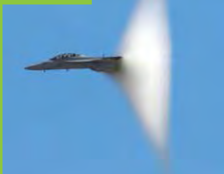
Condensation shock associated with local supersonic flow.
